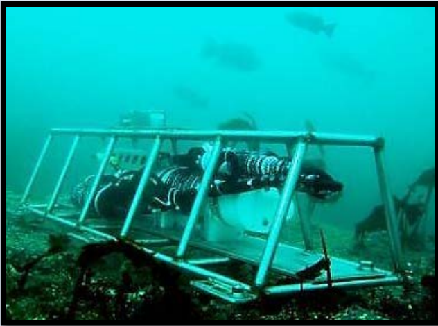
Oceanographic instrument (CTD) bolted to the ocean floor collecting data at Redfish Rocks.
