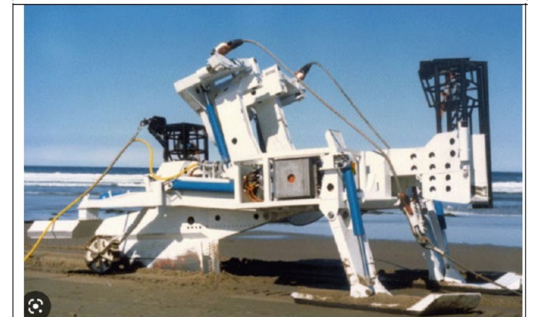
Fiber optic cable plow (source: submarinenetworks.com)
