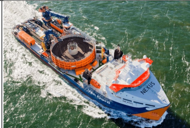
Dedicated power cable installation vessel (source: thenavalarch.com )
