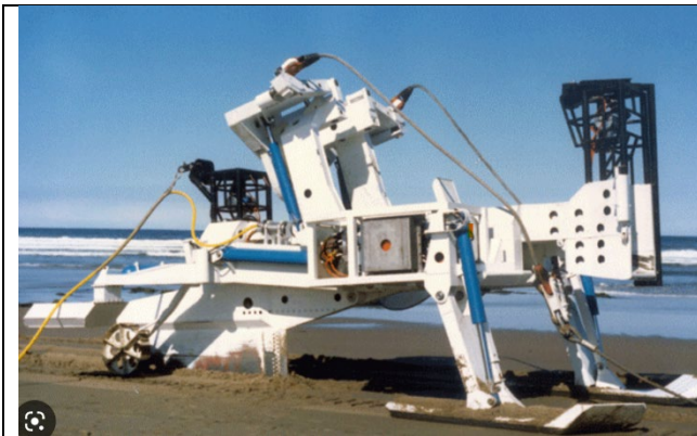
Fiber optic cable plow (source: submarinenetworks.com )
