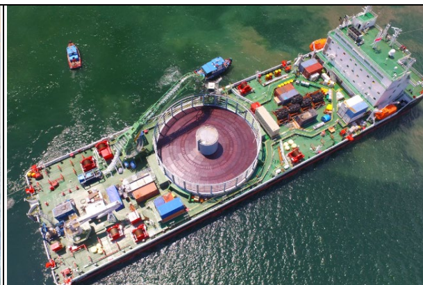
Modified power cable installation barge (source: offshorewind.biz)
