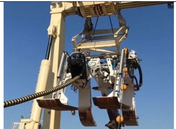
Power cable plow (source: subsea-rov.com )
