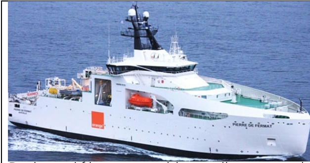
Dedicated fiber optic cable installation vessel (source: iscpc.org/information/cables-hips-of-the-world )
